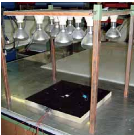
Fig. 3: Test equipment. The panel with the thermocouples is put underneath 10 bulbs of 150 Watt power each. After lighting the bulbs, the temperature of the panel as a function of time is recorded. The sunlight intensity may be varied by varying the distance between bulbs and panel.
