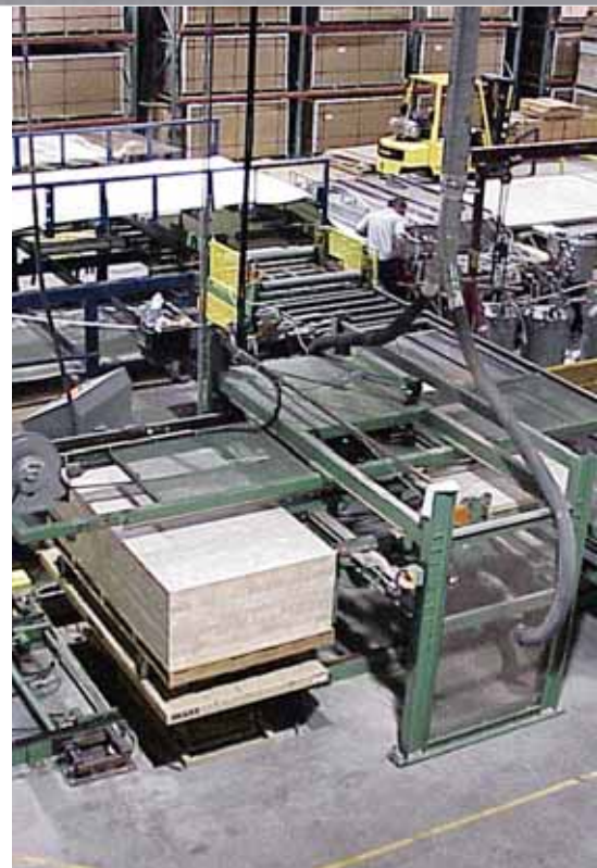
Automated balsa core trim and feed line of Glasforms Inc.
